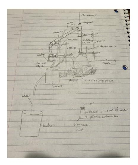
To finish distilling and test the fuel:
